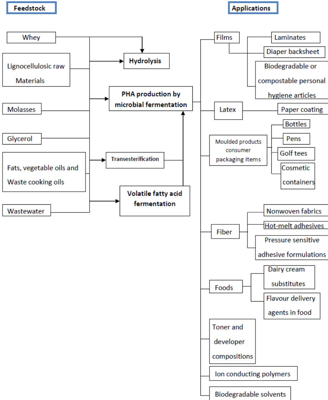
**Figure 3: Feed stocks and applications of microbial PHA productions by different processing technologies**
